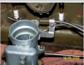
Pull your cables through the bracket, but don't tighten untill after we have the cables connected to their original locations
