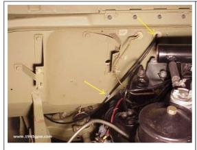
After connecting the cable to the speedometer, run the cable out the firewall and locate the clip that holds the speedometer cable. Then run the remainder down to towards the transfer case as shown.
