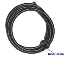
The picture shows the speedometer cable which should be lubricated prior to connecting and routing. The inner speedometer cable can be pulled out of its casing in order to lube, but don't pull it out all the way. You should lube all but the top 12 inches next to the speedometer (Pete Silfven tip) with a light white lube. Any closer to the speedometer and the grease may work its way into the speedometer.
