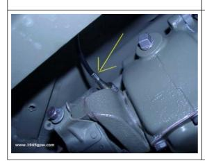
When you are down under your frame, you run your cable through the closest frame hole and back out to the transfer case and connect as shown.
