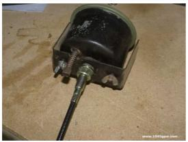
Insert the cable into the back of the speedometer. Then run the other end of the cable out the firewall (shown in next image). Pull the cable all the way out and tighten the speedometer bracket into the dash.
