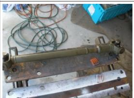
Pete Silfven tip: Make sure the driveshaft is phased correctly so the yokes line up with each other when assembling the slip joint. Also, make sure that the two free cups seat down between the tabs on the pinion flange.
